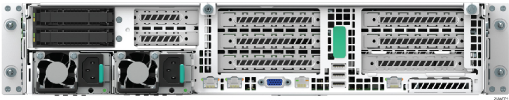
Figure 16. 2U System back panel with optional 2 x 2.5" hot swap drive bay
