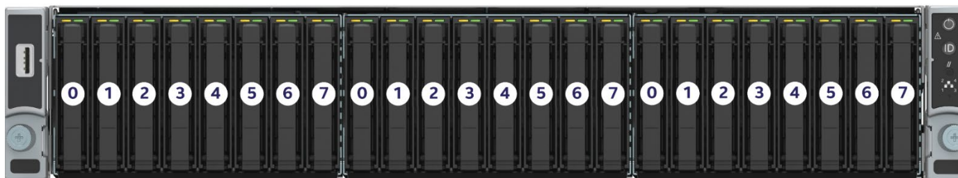
Figure 33. 2U 2.5" drive identification for each drive bay
