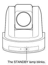
If the camera is moved forcibly, or a finger or other object interferes with camera movement, the camera may fail to memorize the pan/tilt position.
