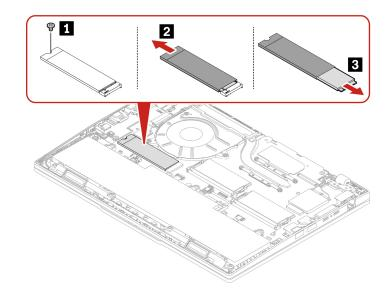
Step 2. Install the 2280 M.2 solid-state drive in reverse order.
