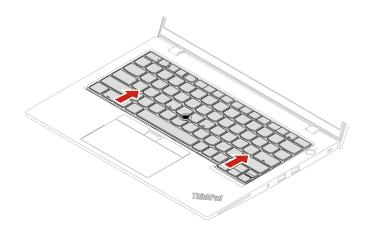
Step 3. Pivot the keyboard slightly upward **1** and then turn over the keyboard **2**.
